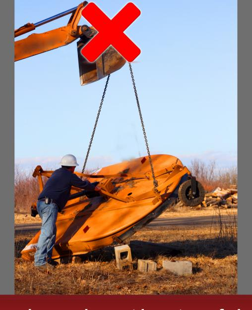
Earth moving equipment is not a safe hoisting device. Earth moving equipment not engineered and equipped with safety devices is a hazard for anyone rigging to it. Cranes are equipped with safety devices designed for hoisting.
