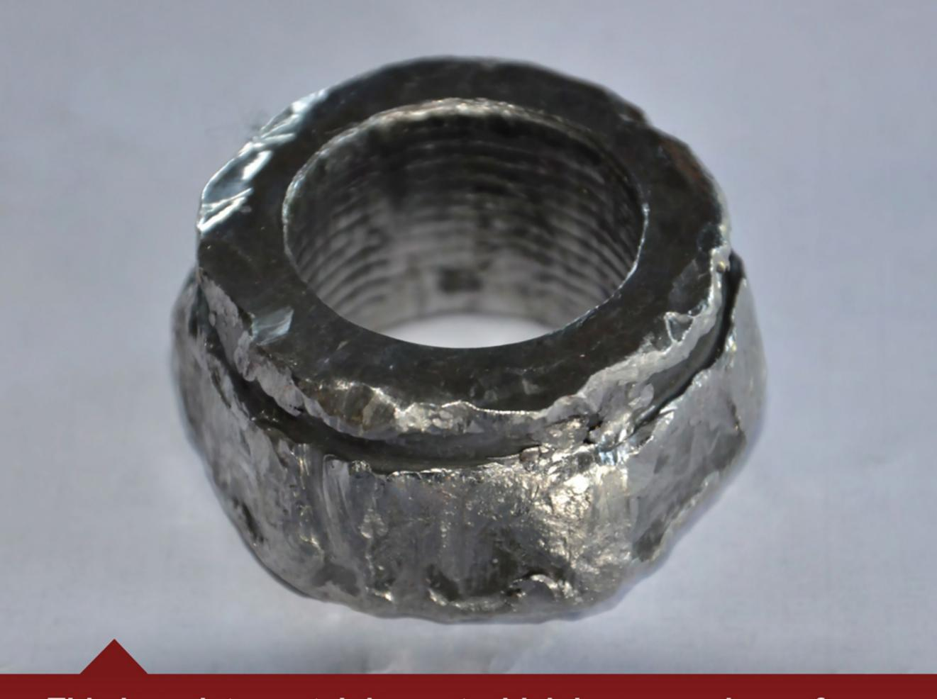
This is a piston retaining nut which has come loose from a hydraulic cylinder. The nut was destroyed by the piston before the rod assembly left the cylinder barrel. When a hydraulic cylinder comes apart it can be a catastrophic failure. Correct nut torque may be only part of the full procedure.
