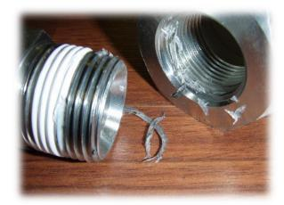
Thread sealant can become a contaminant if not applied correctly and cleared when disconnecting and reconnecting.
