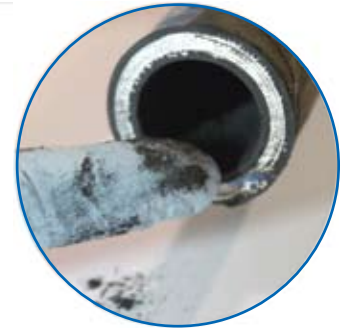
Debris from the cutting process or other foreign objects may contaminate your system.
