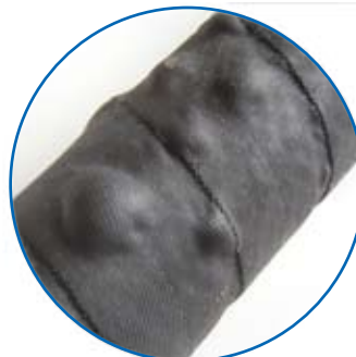
Hydraulic Hose Blistering indicates a failing hose which could rupture at any time.
