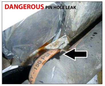
The source of the leak and the fluid streaming from it may be very small and not easily visible. It is important to only use the far end of a long object such as a piece of cardboard or wood in the suspected path of any fluid stream.
